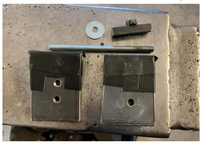
5) Rivet the threaded rod into place. Could also be welded and afterwards ground.
